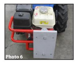
Using the same method as described above, the Kit can be installed vertically on the red wrap-around bumpers utilizing the top and middle tubes (Photos 4 - 6). This helps center the Kit directly in line with the tractor, but there's no significant performance advantage from the method above. The angle of the brackets to accommodate the platers are secured by two 17mm wrenches.
