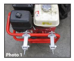
First, install the brackets using the bolt pattern on the weight plates as a guide to achieve proper spacing between each bracket (Photo 1). The curved end of the brackets fit around the tubular bumper and are fastened with two 13mm wrenches.
