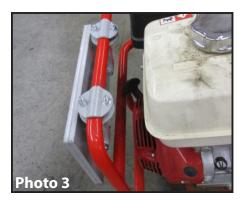
The brackets can also be collapsed (Photo 3). This negatively alters the tractor's fulcrum point for heavy rear-mount attachments, but provides better clearance for the operator's legs if installed during front-mount (mowing) mode.
