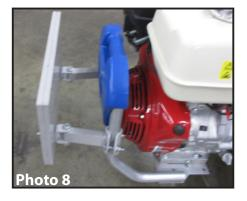
**NOTE:** Each weight plate features three rows of bolt holes. For black/ silver bumpers, we recommend using the bottom row of holes for sufficient ground clearance (Photo 8).
