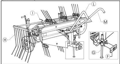
Before being used, the rake tedder must be lubricated by greasing (Vedi 4.5)
