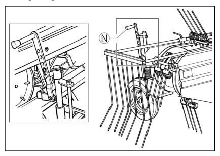
The machine is adjusted always operating on the wheels uprights by moving the handle (N).
