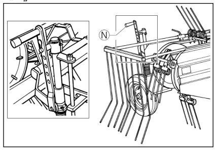
For raking the lever (N) must be in the indicate position.
