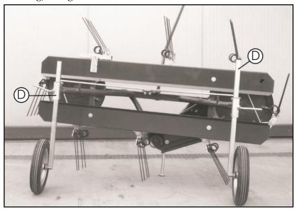
The machine is adjusted always operating on the wheels (D) as showed in the picture.
