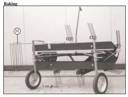
The band runs horizontally and must be adjusted about  $1\div 2$  cm above the ground so that fodder is raked up without causing excessive stress on mechanical parts.
