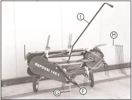
Before being used, the rake tedder must be lubricated by greasing (Vedi 4.5)
