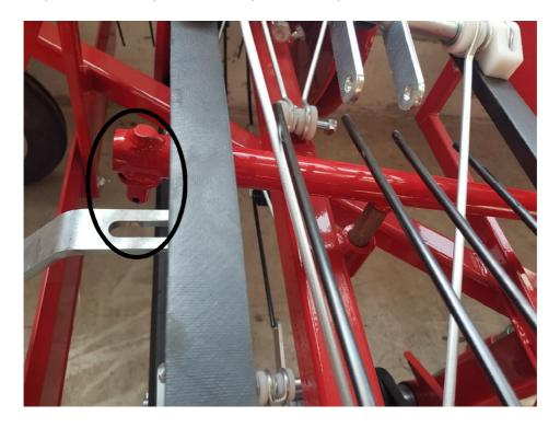
Fix the rudder with the split pin and the screw (do not forget the washer!) previously removed.
