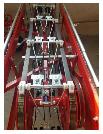
Turn each pair of springs in its position and fix it through the bolt as depicted in the following picture.
