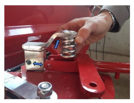
Fix the red rod to the zinc cube with screw, washer and bolt (see the above and below pictures)
