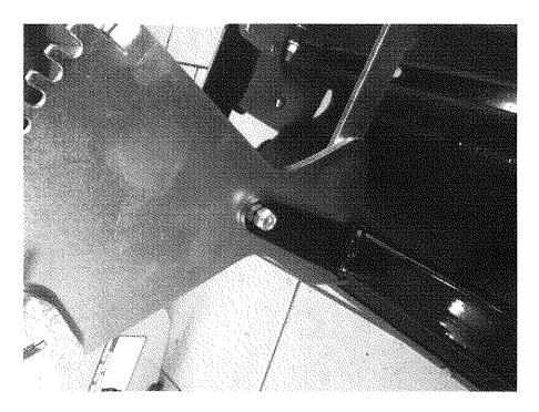
Install the 5/16 bolt on the lever part and firmly tight It.
