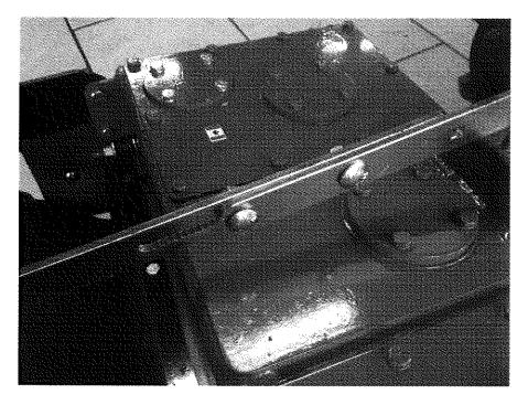
The two carage Bolt on the middle of the arm require a final ajustement to be able to completly lift the implement.
