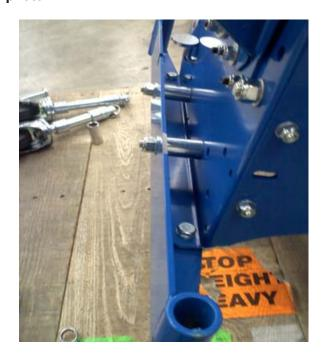
• After the front axle is on, tip the unit forward and install the two large blue mounting brackets onto the body of the unit. Next put the two belts on the driven, (small) pulley set and thread them onto the drive (large) pulley set. Now snug the four large cap screws that fasten the pulley set to the two large brackets and pry down on the pulley set to tighten up the bolts.
